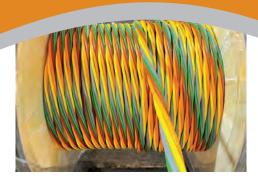
Priority-Plex® takes your multiple single reel RW90 conductors, and twists them at the factory making them handle like a single cable. Priority-Plex® cables have a smaller/unified diameter than parallel which makes pulling them easier and faster. One pull vs multiple pulls with single reels can result in over 50% labor savings.
